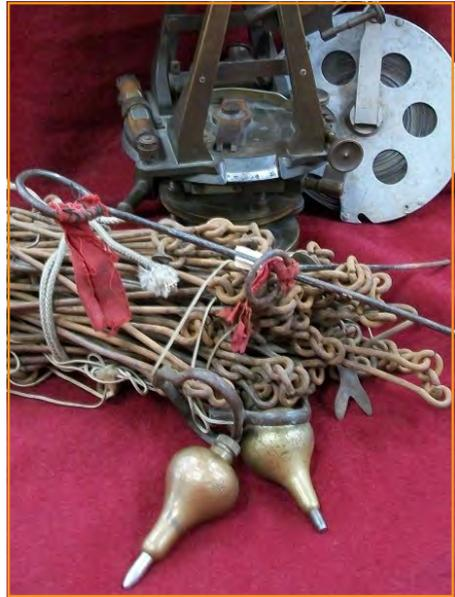
Throughout recorded history surveyors have used many devices for measuring distances. These devices have included rope, poles, grape vines, pacing, steel tapes, electronic devices and "chains". The basic "Gunter's" chain was the primary tool of surveyors to measure distance in North America from the 1600s to the end of the 1800s. The basic idea of a chain is to be 66' long with 100 links making up the chain.
