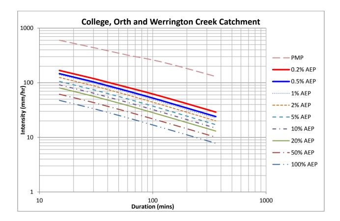
The 0.5% AEP and 0.2% AEP intensities were subsequently extracted from the chart for a range of durations:
