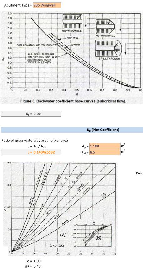
K<sub>p</sub> = σΔK K<sub>p</sub> = **0.40**  Pier Type: Dual Square Pier
