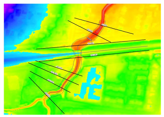
Plate P1: HEC-RAS model cross section layout and DEM in the vicinity of the railway culverts and embankment
