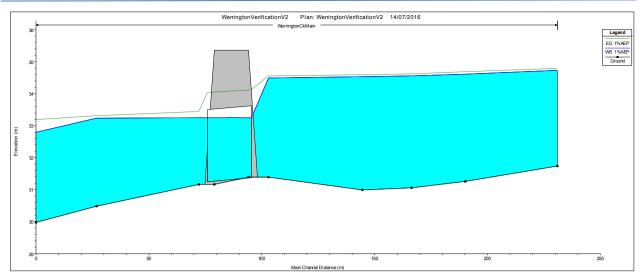
Plate P4: Peak 1% AEP Stages for the Railway culverts on Werrington Creek
