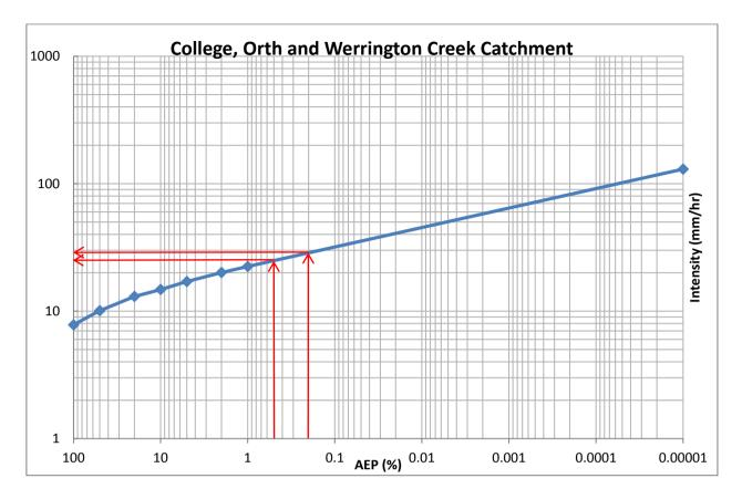
6 hour rainfall intensities for the 0.5% AEP and 0.2% AEP event were extracted from the above chart. This produced the following 6 hour intensity values:
