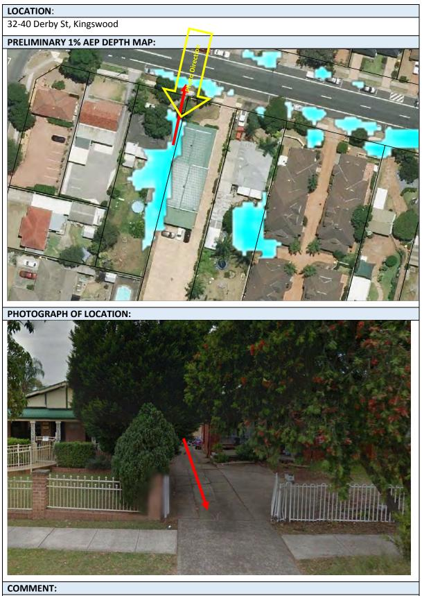
Water from rear of no 40 can easily pass down driveway to Derby Street. Remove from Mapping.
