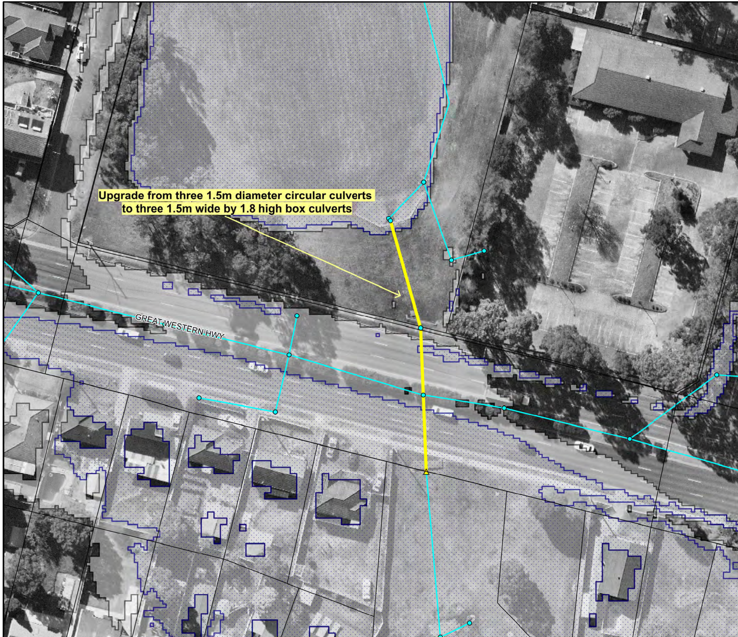
Figure 57: FM1: Great Western Highway Culvert Upgrade
