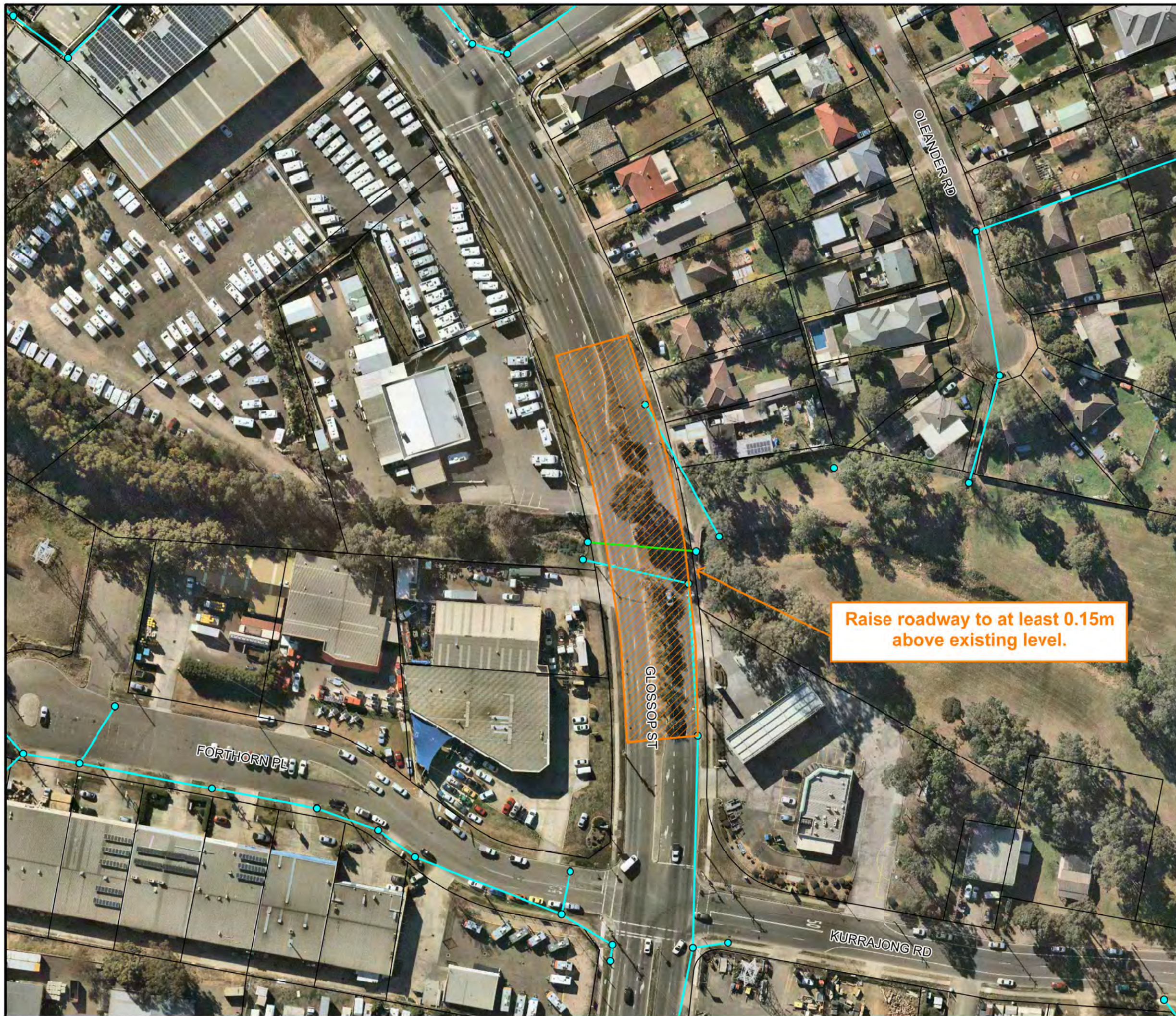
Figure 67: RM9: Glossop Street Roadway Modification
