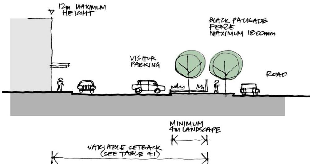
Figure D3.3: Illustration of Building Setbacks – Larger Site (Plan View)
