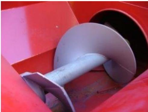
Figure 31: Integrated Auger used to compact objects within the compaction unit
