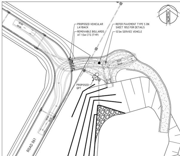
**Figure 8-13 Basin B Maintenance Access**
