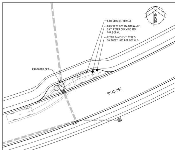
**Figure 8-3 Stage 1 Road 009 GPT Maintenance Access**
