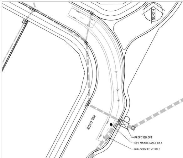
**Figure 8-6 Stage 2 North Road 071 GPT Maintenance Access**
