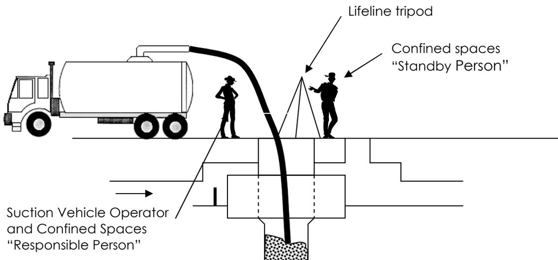
NB: A person may be needed inside the CDS unit to guide the head of the suction hose.
