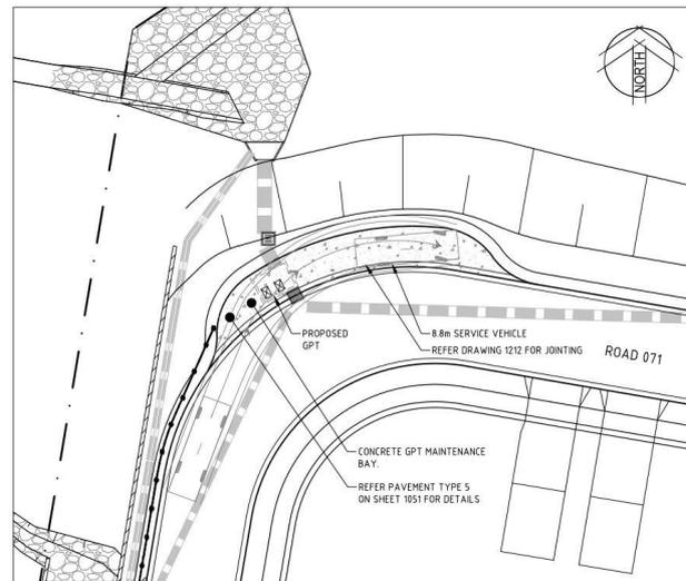
**Figure 8-7 Stage 2 Road 002 & 070 GPT Maintenance Access**
