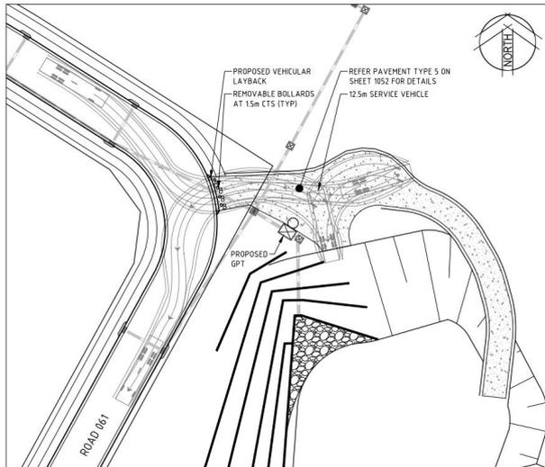
**Figure 8-9 Stage 1 Road 064 GPT Maintenance Access**
