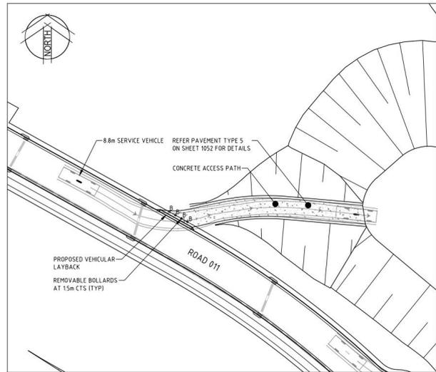
**Figure 8-14 Basin D Maintenance Access**
