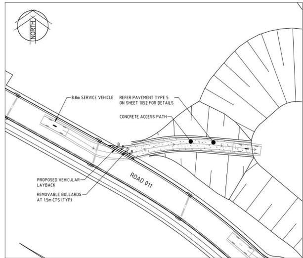
**Figure 8-14 Basin D Maintenance Access**
