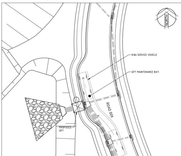
**Figure 8-4 Stage 1 Road 011 GPT Maintenance Access**
