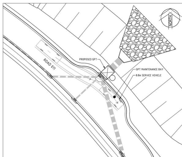
**Figure 8-5 Stage 1 Road 060 GPT Maintenance Access**
