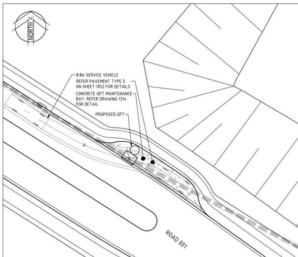
**Figure 8-2 Stage 1 Road 002 GPT Maintenance Access**
