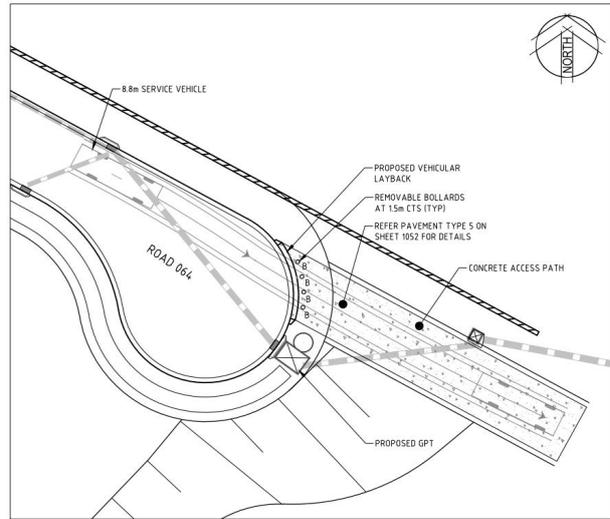
**Figure 8-10 Stage 2 South Road 071 GPT Maintenance Access**
