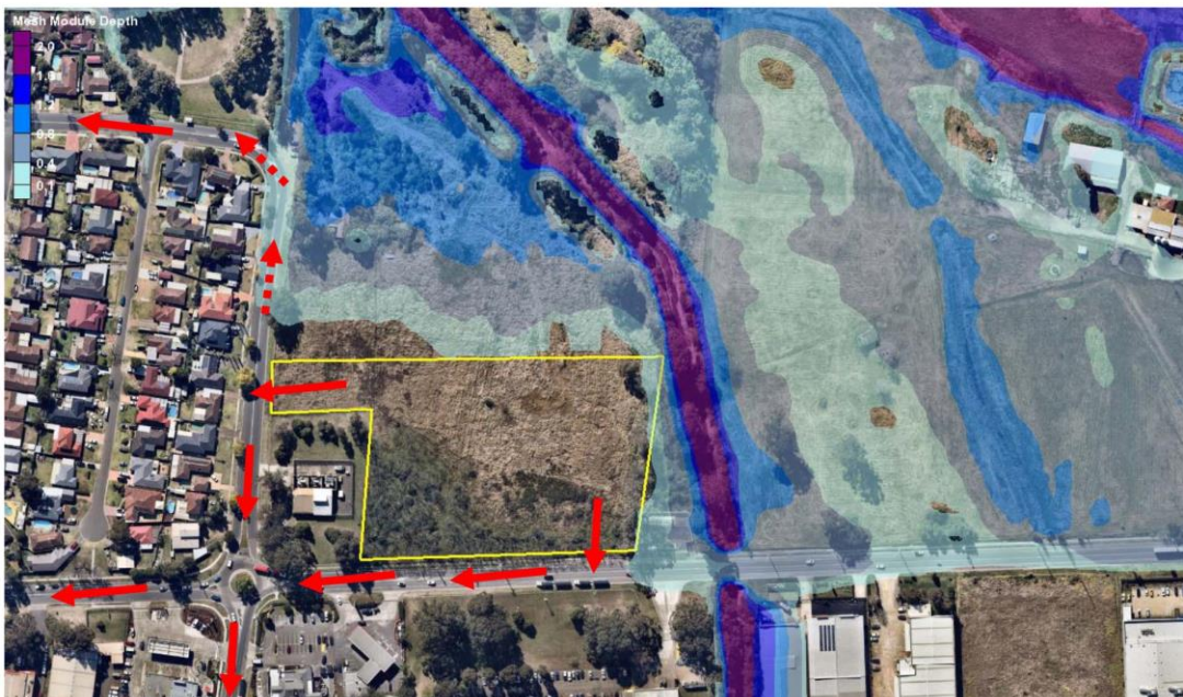
Figure 5.3-1 1% AEP Post-Development Flood Evacuation Routes
