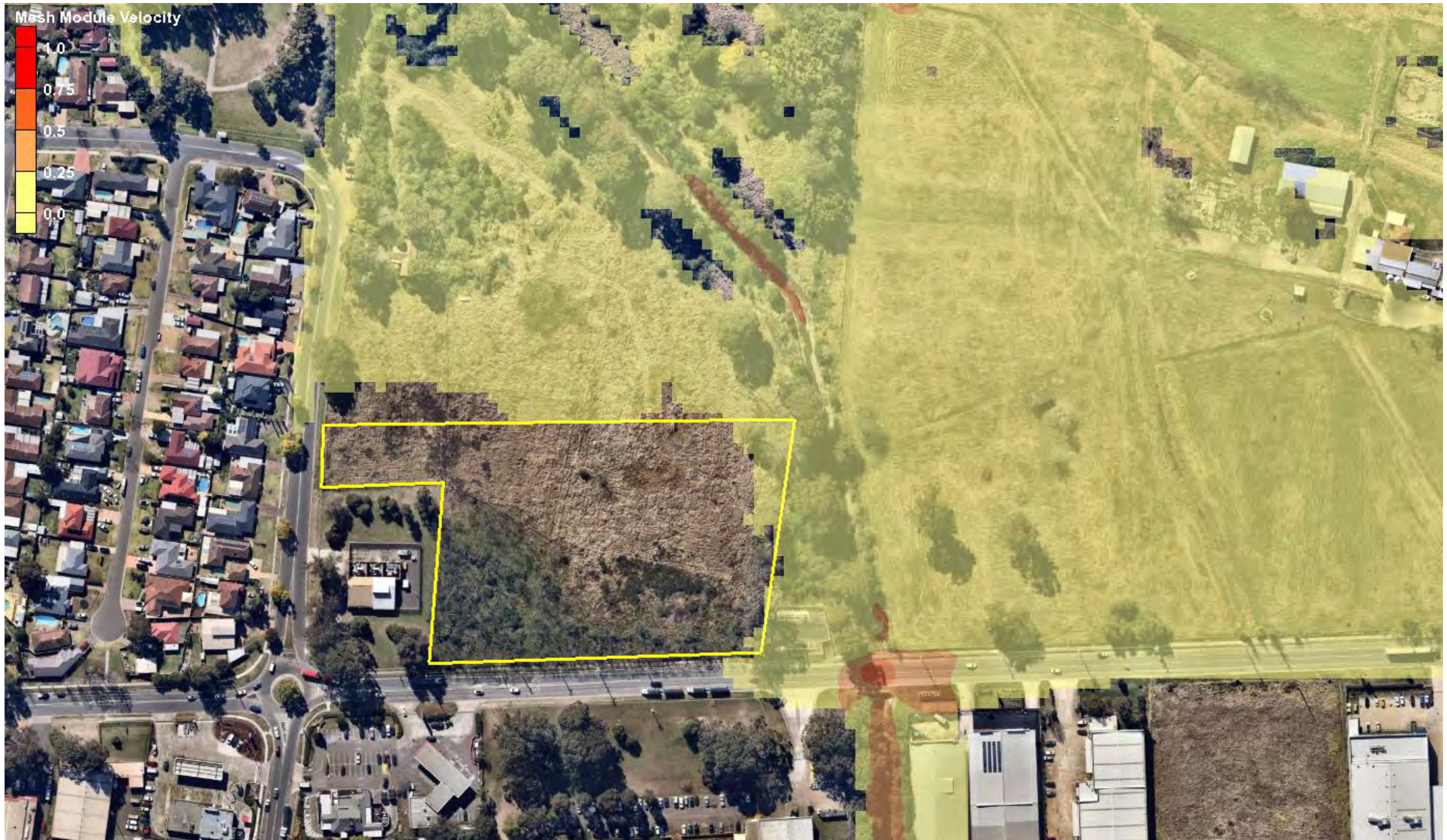
Figure B2.3: 1% AEP Flood Velocity – Post-Development
