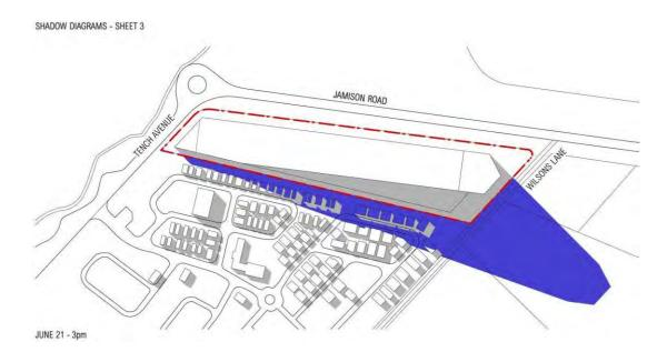
Figure 13.17 Shadow diagrams generated by the indicative building envelope showing maximum extent of shadow
