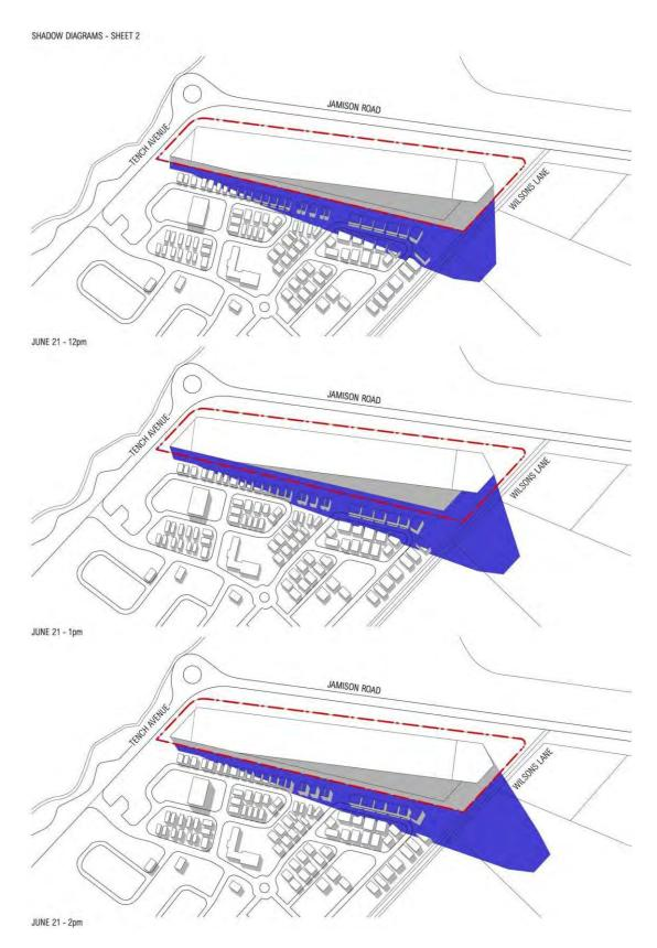
Figure E13.16 Shadow diagrams generated by the indicative building envelope showing maximum extent of shadow
