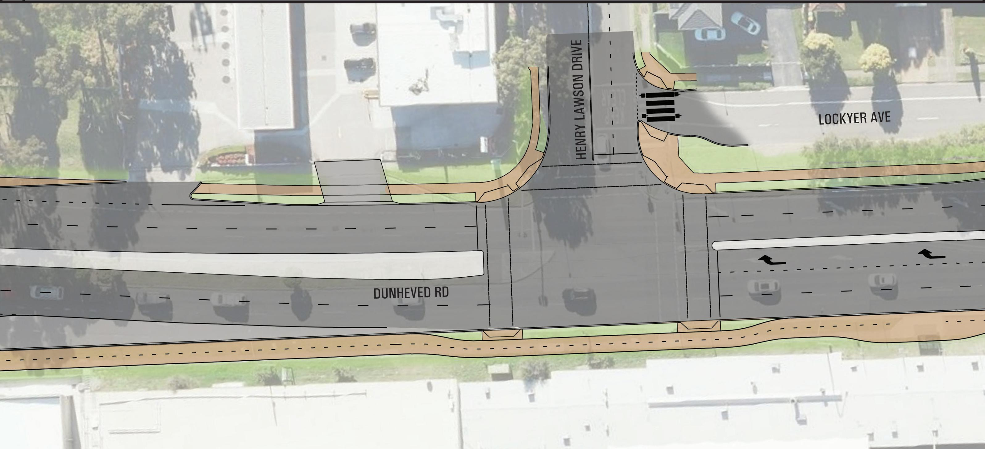
New four lane carriageway and upgraded signalised intersection. Removal of pedestrian zebra crossing and partial closure to Lockyer Avenue to simplify the intersection. Vehicles will now exit Lockyer Avenue at John Batman Avenue.
