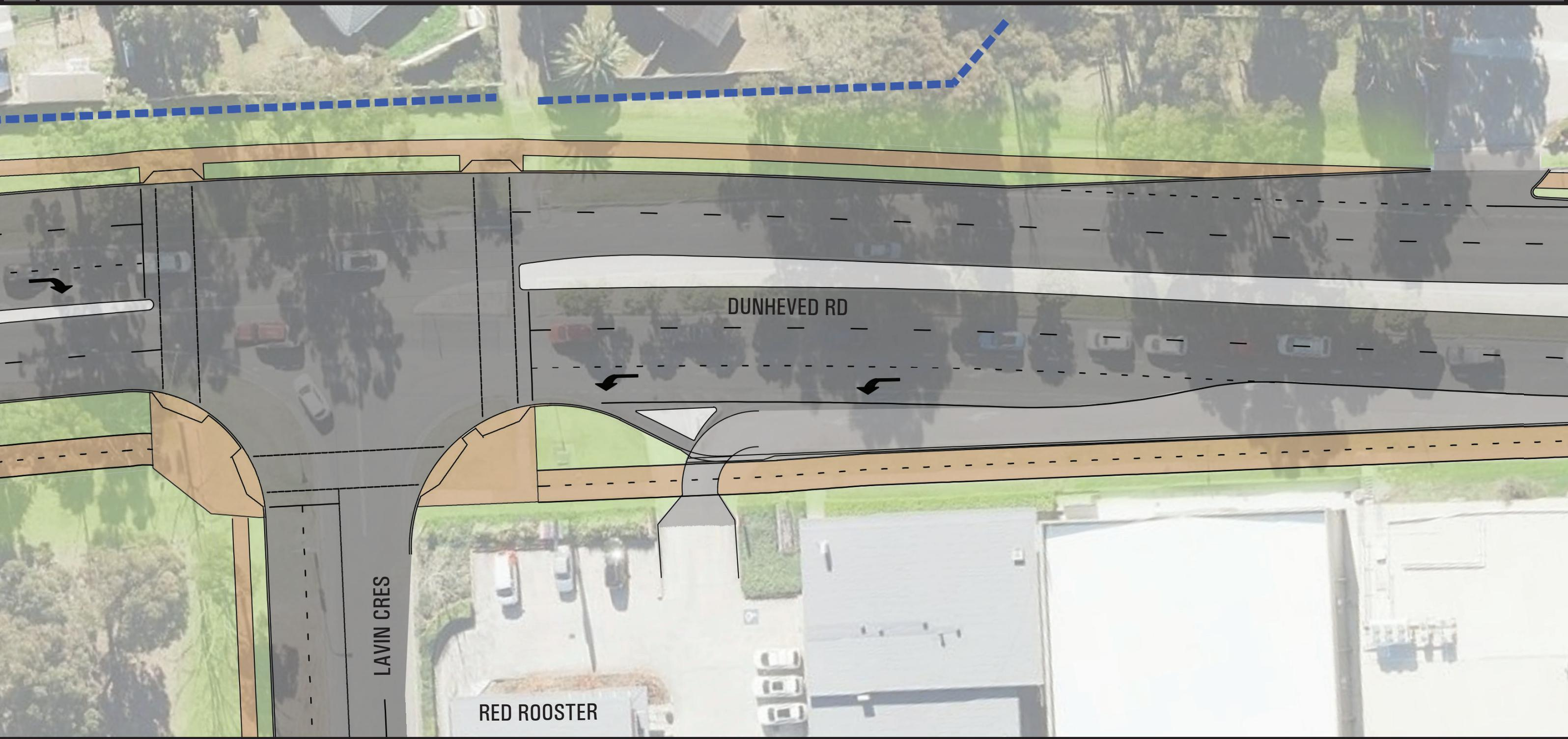
New four lane carriageway, new signalled intersection and maintain left lane into shopping area with a 400mm wide median separator
