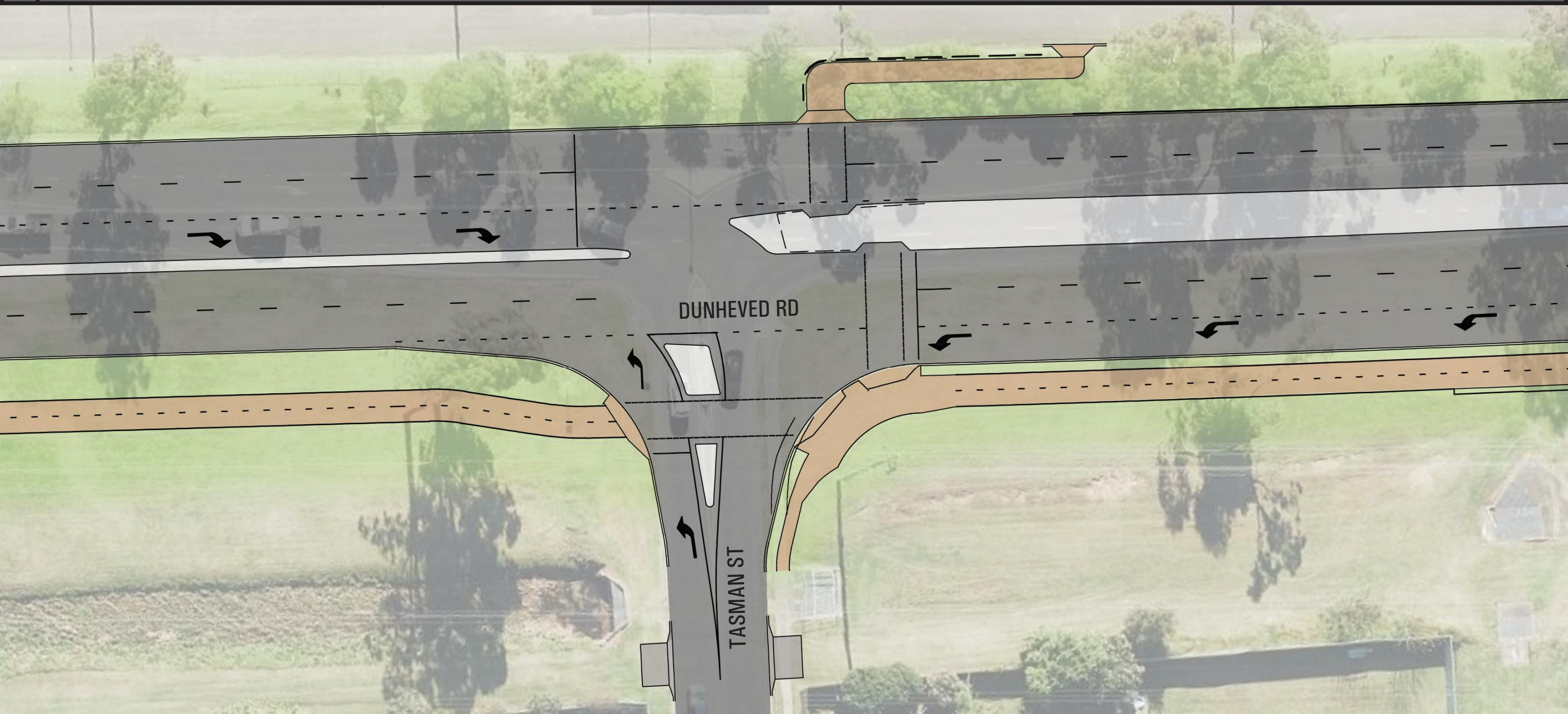
New four lane carriageway and signalised intersection with right turn permitted into Tasman Street and the current westbound left in / left out access maintained for Tasman Street. New signalised pedestrian crossings for Dunheved Road and Tasman Street. Eastbound access to Dunheved Road from Cambridge Park will now be via the upgraded traffic signals at Francis Street
