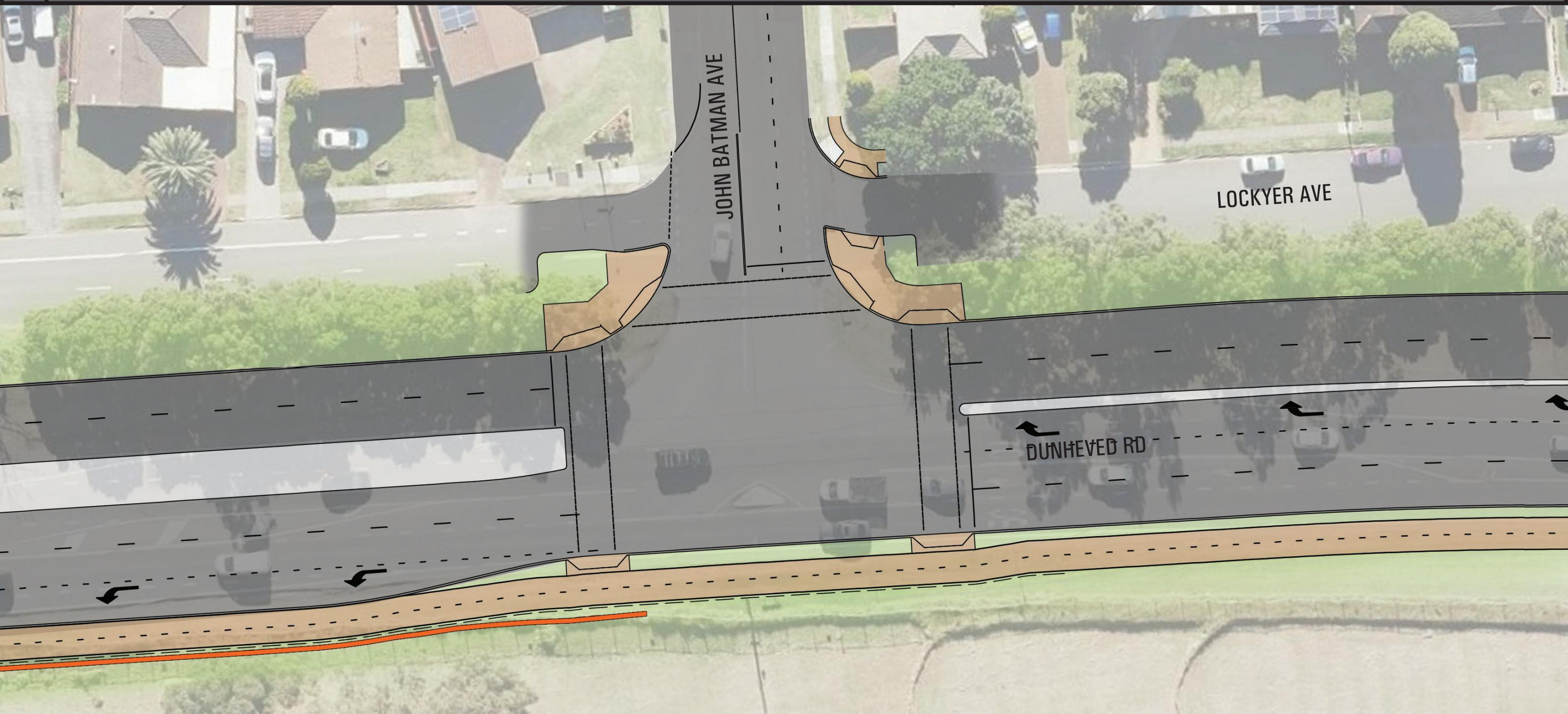
New four lane carriageway and new signalised intersections. Partial turn closures to Lockyer Avenue to reduce vehicle conflict. New single lane roundabout to Ovens Drive at John Batman Avenue to assist with residential access to and from Lockyer Avenue.
