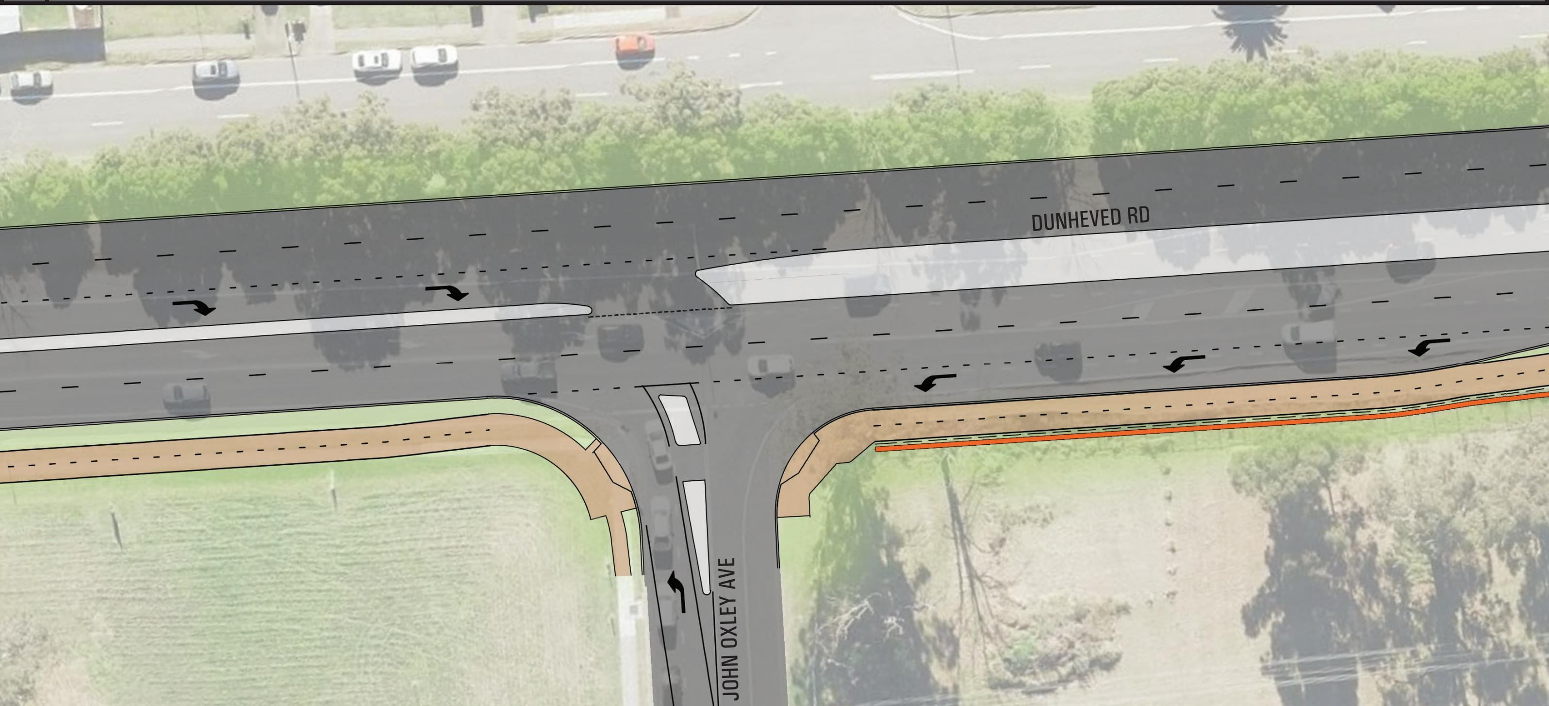
New four lane carriageway and upgraded intersection. Upgraded intersection with right turn permitted into John Oxley Avenue and the current westbound left in / left out access maintained for John Oxley Avenue. Safer eastbound access to Dunheved Road from Werrington will be via upgrade traffic signals at Francis Street or via the Parks Avenue and Werrington Road intersection.
