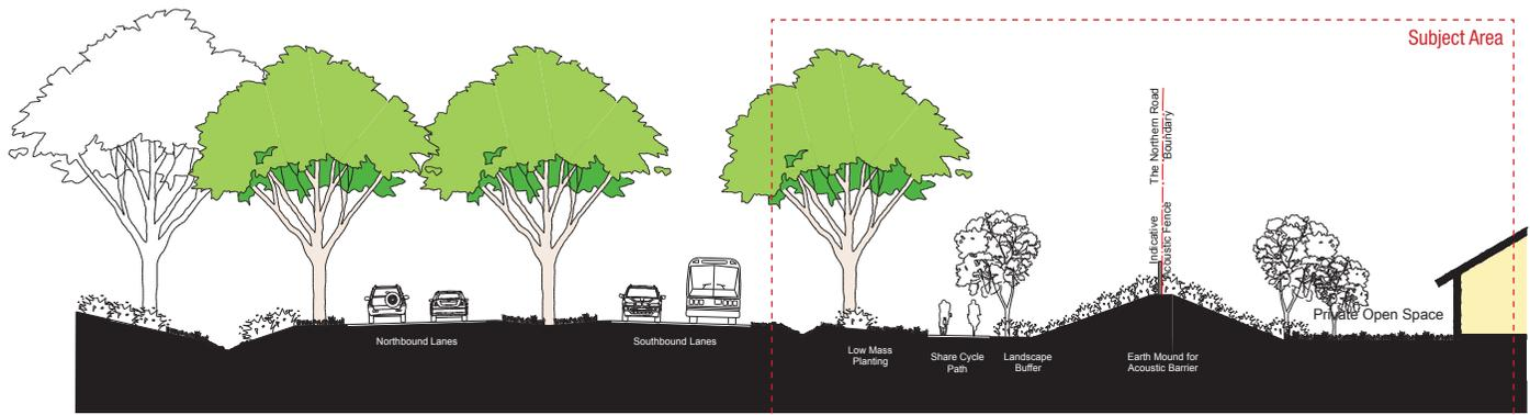
OPTION A: Section of The Northern Road – Acoustic Barrier and Earth Mound
