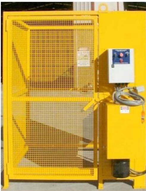
Figure 32: 1100L bin lifter used to empty bin into the Auger Compactor
