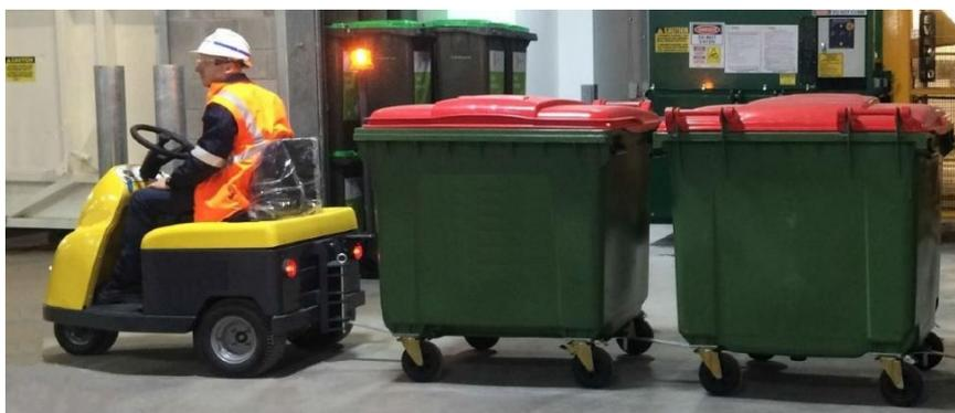
**Figure 16: Universal Towing Device pulling 1100L bins behind an Electric Tug Device**
