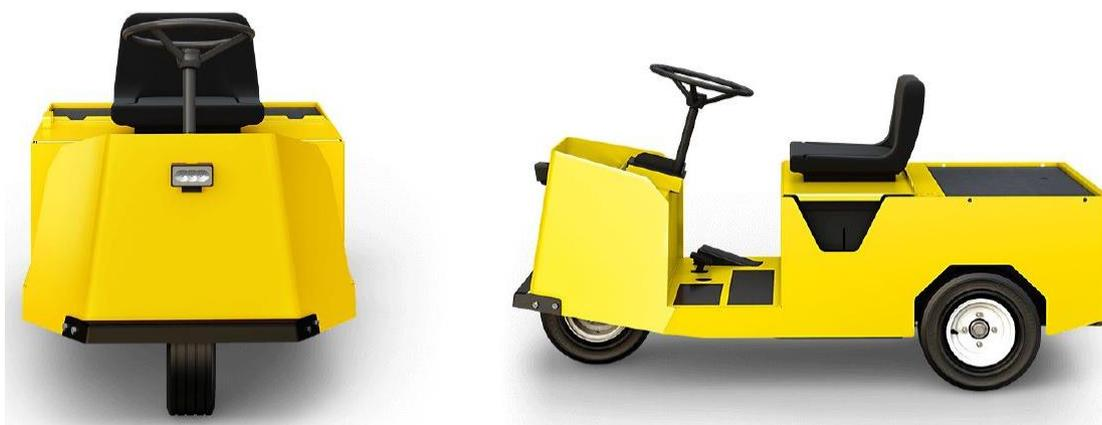
**Figure 11: Typical Electric Ride On Tug Device used by the caretaker for the movement of 660L & 1100L bins within the development**
