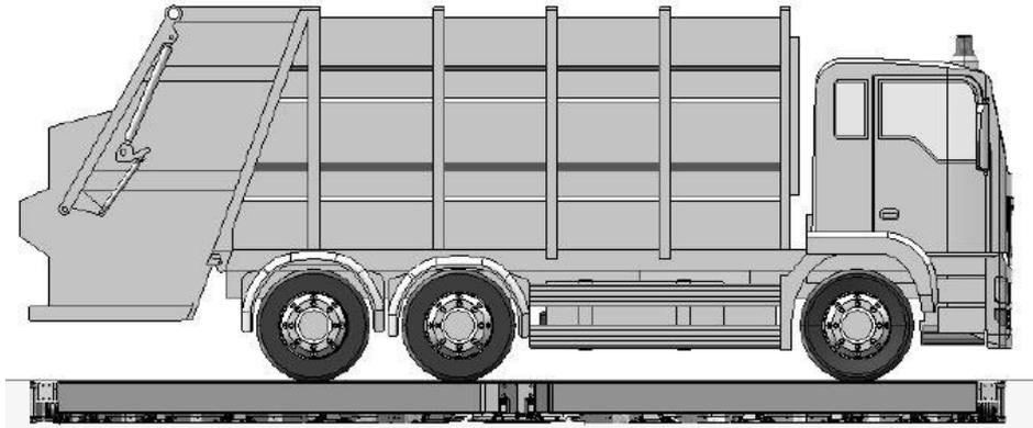
**Figure 6: Correct vehicle loading alignment showing central alignment and no vehicle overhang**
