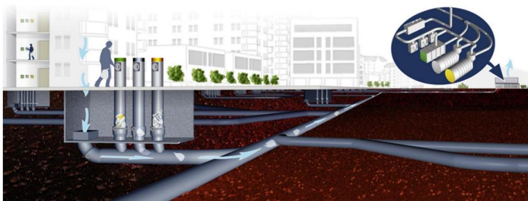
Figure 56: Schematic of the Automated Waste Collection System
