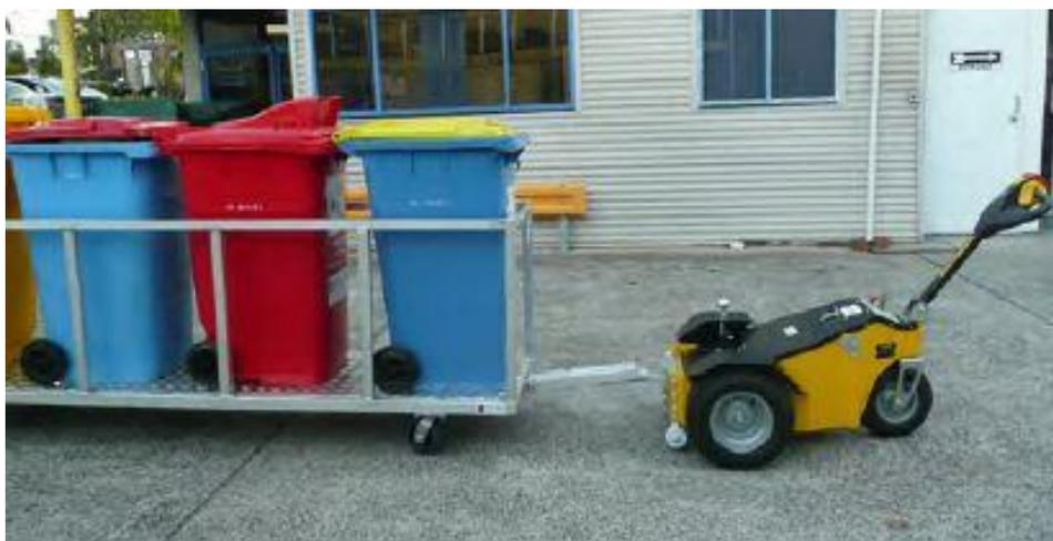
**Figure 22: Portable Bin Tug Device moving bins using an aluminium trailer**
