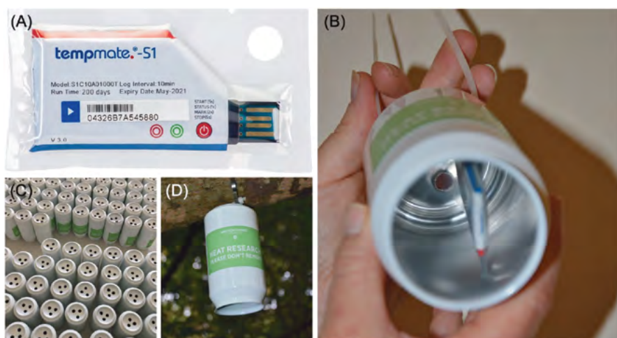
FIGURE 3: Details of the Local Heat Logger designed by Western Sydney University. (A) The sensor used to record near-surface air temperature. (B) The protective shield with sensor inside. (C) Detail of the shield showing the holes necessary for air flow inside the shield. (D) Installation of the Local Heat Logger in the field with the open bottom facing the surface.
