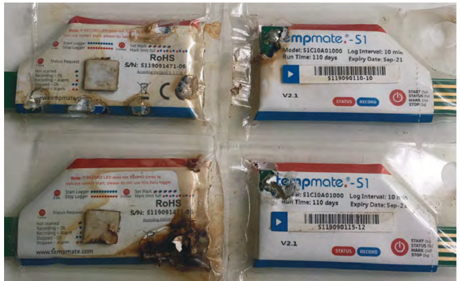
FIGURE 6: Sensors that showed signs of electrical and/or physical damage after being deployed in the field for several months. Data from all damaged loggers were retrieved without problems.
