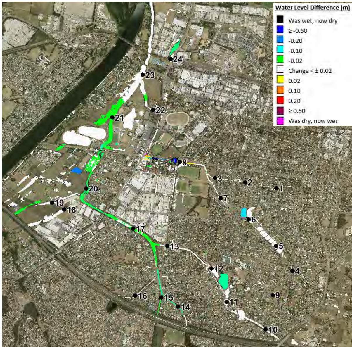
Plate O5 5% AEP Flood level difference map with higher continuing loss rate
