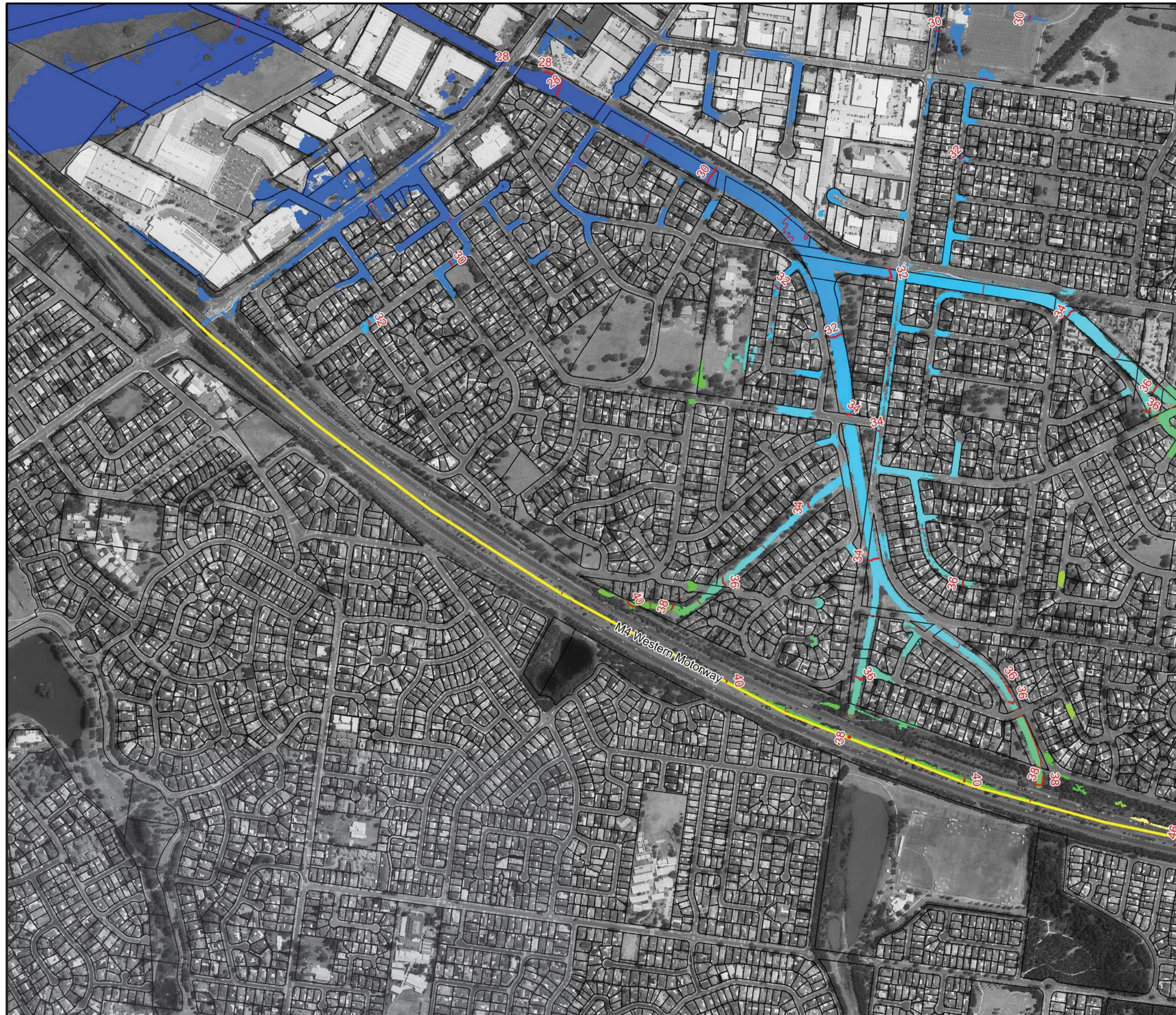
Figure 62.4: Peak Water Levels for the 1% AEP Flood
