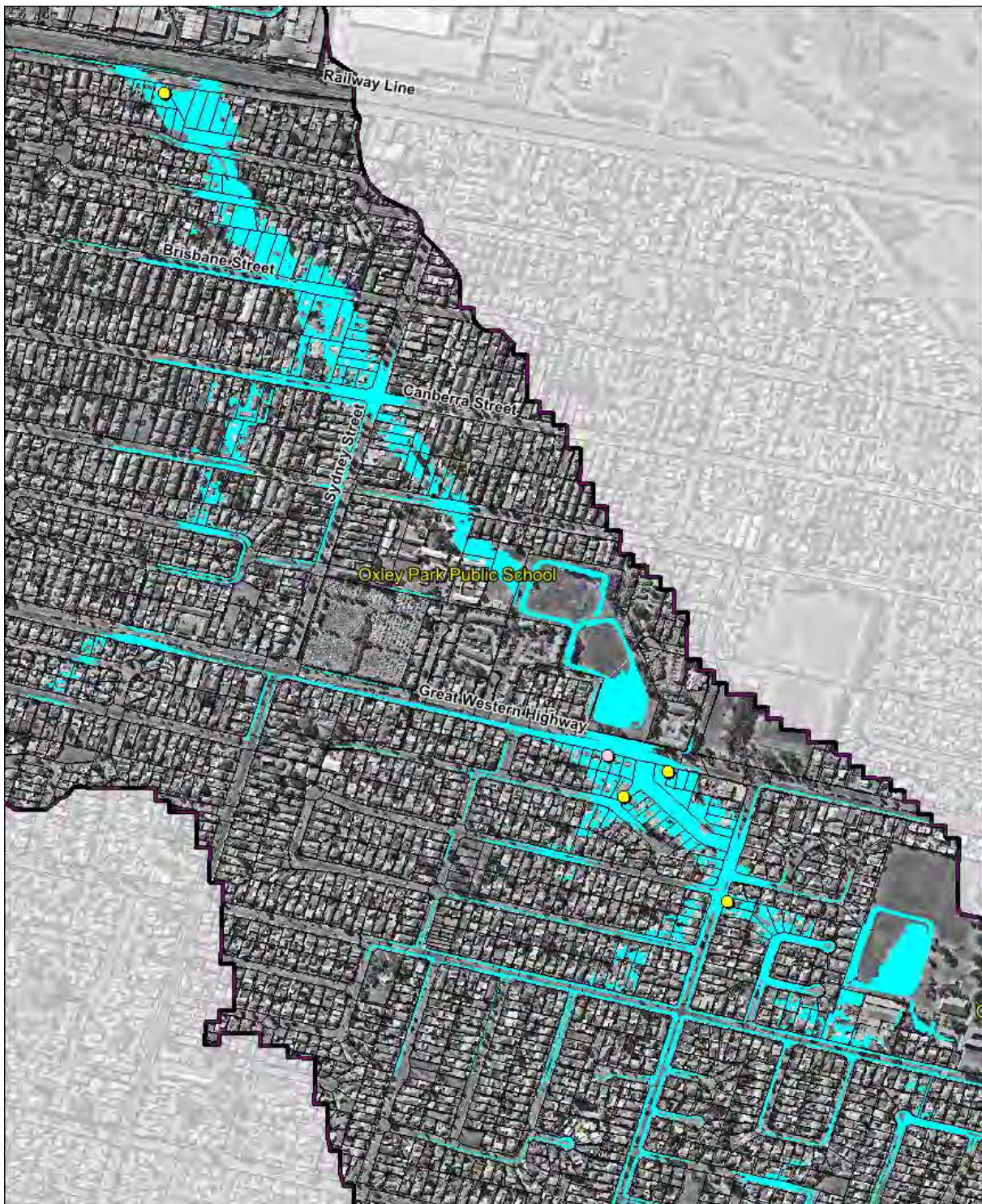
Plate 43 1% AEP low hazard areas (aqua) and properties potentially eligible for voluntary raising (yellow) or voluntary flood proofing.
