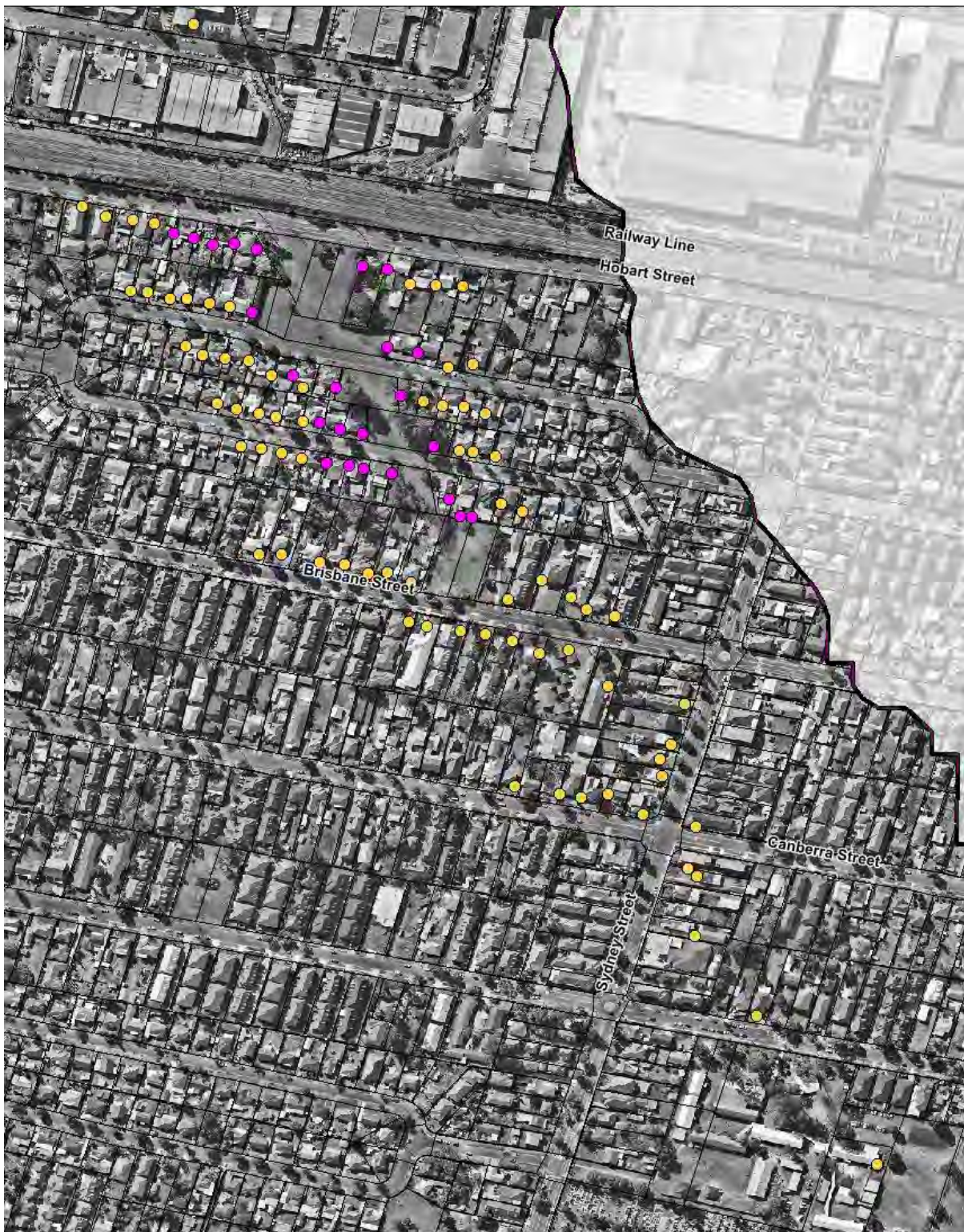
Plate 39 Buildings exposed to H5 (orange points) and H6 (magenta points) hazard during the PMF.
