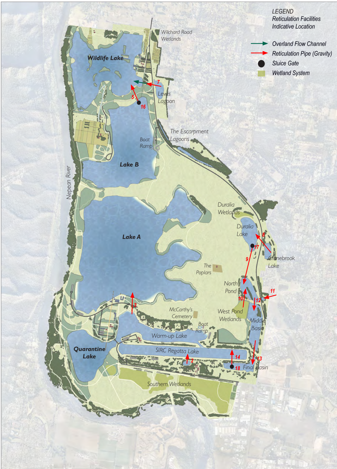
Figure 11: Completed Water Supply and Reticulation Works
