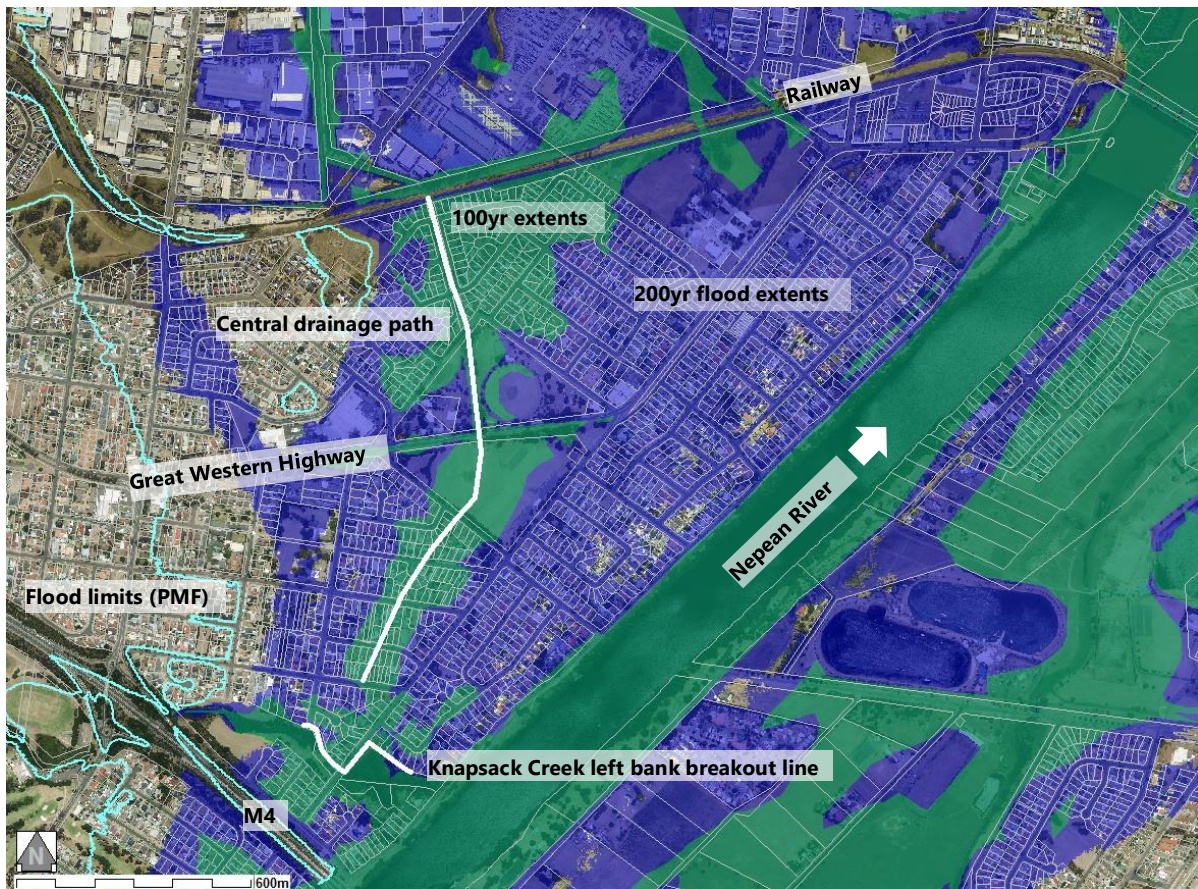
Figure 43 - Emu Plains residential area flood related characteristics
